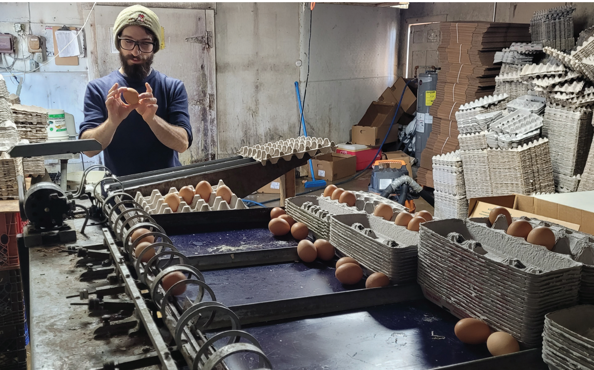
GRADE A: Fourth-generation poultry farmer Adam Baffoni, of Baffoni Poultry Farm in Johnston, still uses a mechanical egg-grader from the 1950s, to sort and grade his fresh farm eggs. He said he has been using the machine since he was five years old. Below, the Rhode Island Reds rule the roost. (Sun Rise photos by Rory Schuler)
